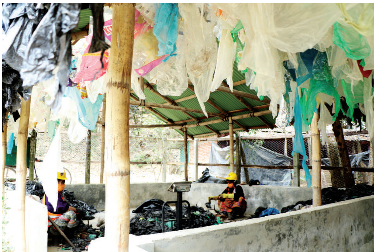
Polythene segregation unit for recycling
